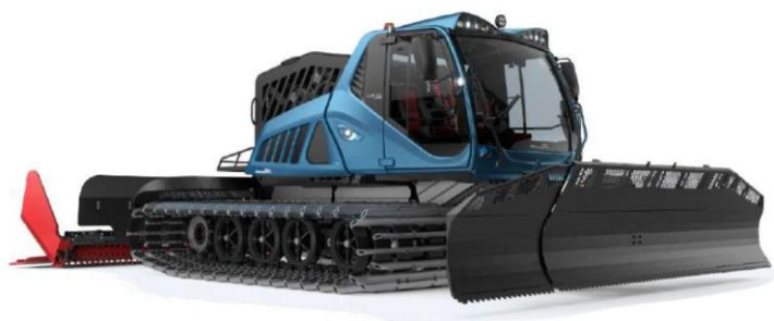
Figure 8. Example of H 2 fuel cell electric snow groomer. Model: Leitwolf H 2 Motion manufactured (prototypal stage) by Prinoth 5 .
