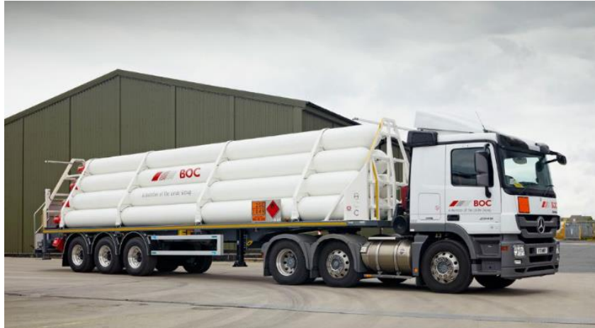
Figure 18. Example of a towed tuber trailer for transporting hydrogen at 250 bar (Cussons, 2019).
