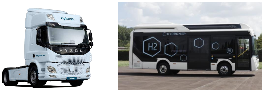
Figure 7. (Left) Fuel cell electric tractor truck by Hyzon 3 . (Right) 13m fuel cell electric bus by Rampini 4 .
