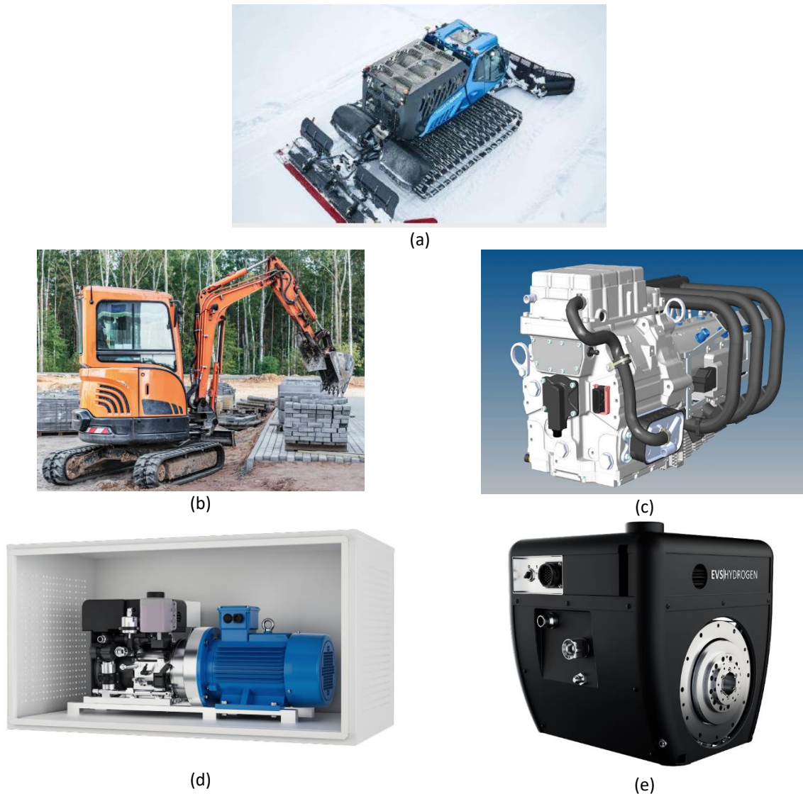
Figure 10. (a) Prinoth H2 ICE snow groomer. (b) Construction machine powered by H2 ICE. (c) H2-based electric vehicle range extender. (d) H2-based recovery drive for electricity and heat from hydrogen storage systems. (e) H2 industrial engine 7 .
