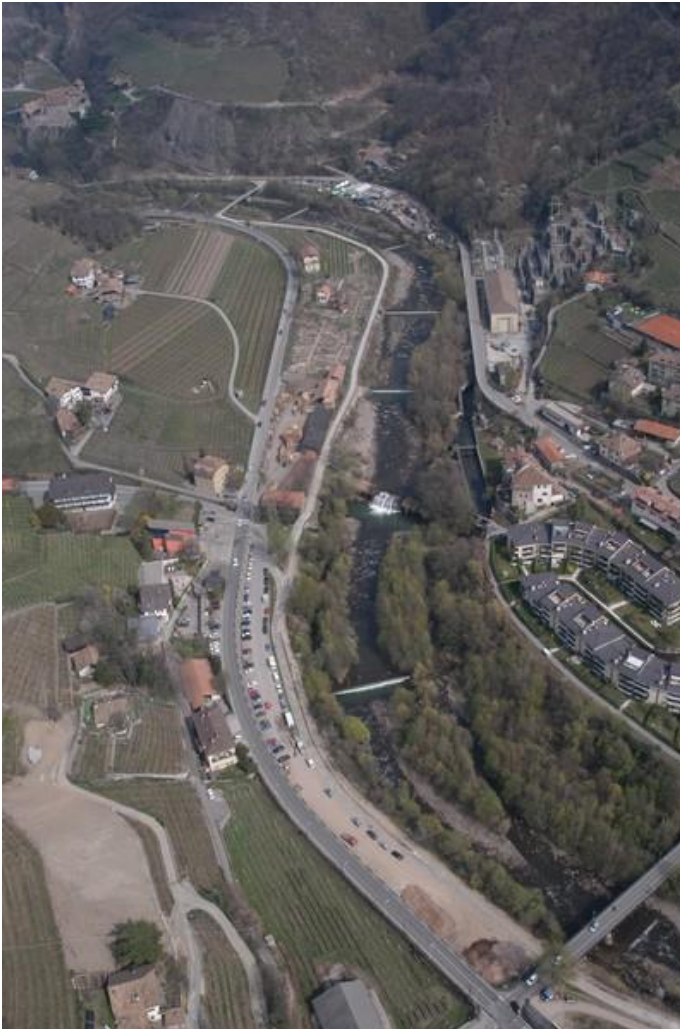
Figure 5 – Upper Talvera river-reach pre-restoration. Series of weirs and a consolidation check dam impeding fish passage. On the orographic left, the S. Antonio hydropower plant.
