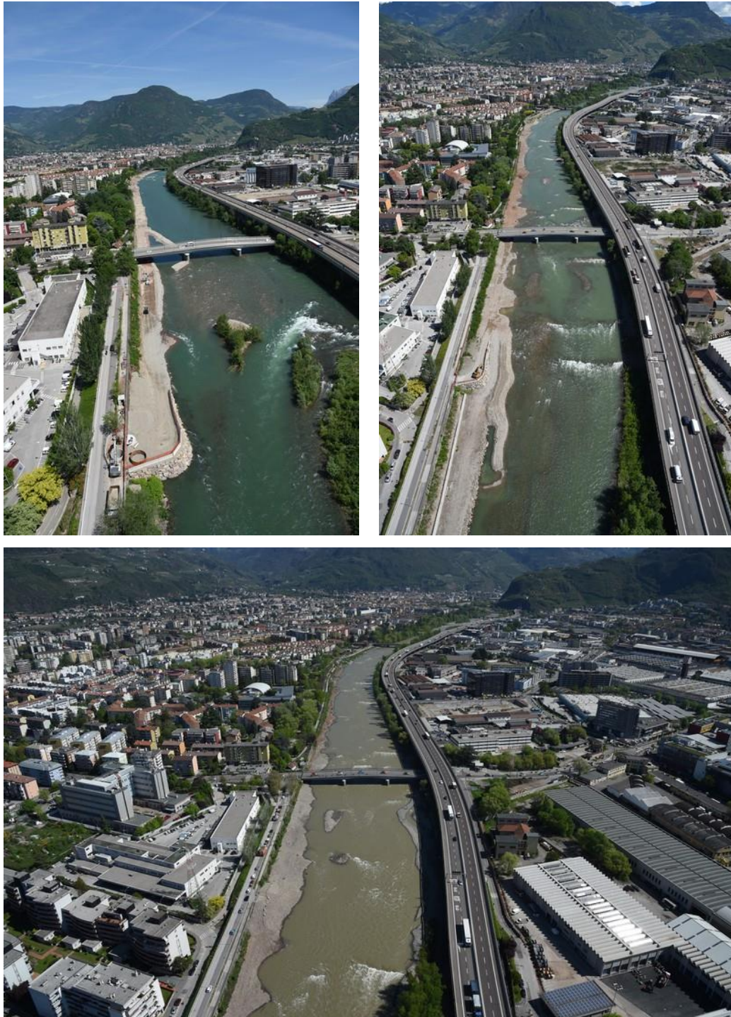
Figure 9 - Isarco River at Resia bridge in 2015 (top-left), 2016 (top-right) and 2018 (bottom). In the most recent pictures flow deflectors are visible as well as riverbanks variability
