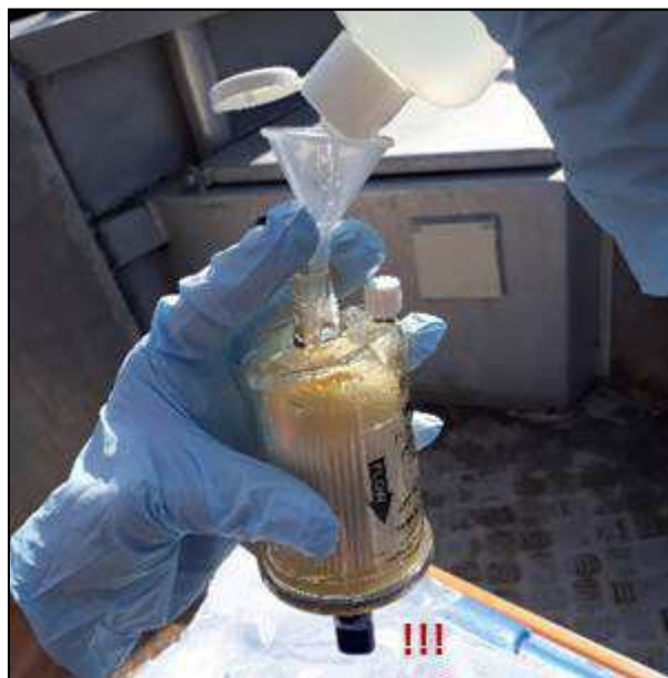
Figure 2. The preservation buffer can be added to the VigiDNA® filter capsule using a small DNA-free funnel. Important: ensure that the outlet of the filter is closed before adding the preservation buffer!!!
