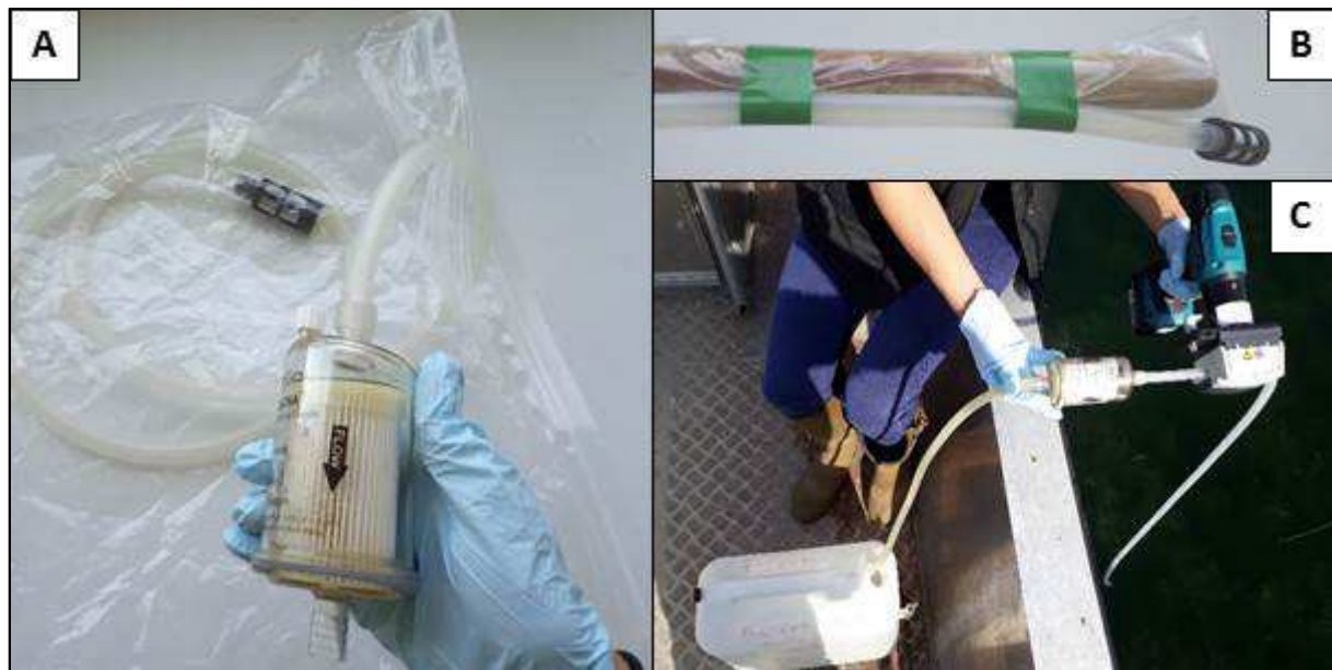
Figure 4. Pictures showing how to: connect the clean DNA-free tubing to the filter cartridge (panel A), attach the sampling tubing to the sampling pole/stick to keep the tube below the water surface while sampling (panel B) and collect and filter water samples for the integrated sampling protocol (panel C).
