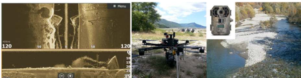
Figure 1. Vectors and sensors usually used for the physical monitoring, from left to right: image from the bathymetric echosounder used in the Lech river (Germany); drone equipped with a LiDAR sensor and a digital camera used on the Buëch and Drac rivers (France); in situ timelapse camera deployed in the Drac river (and resulting image)
