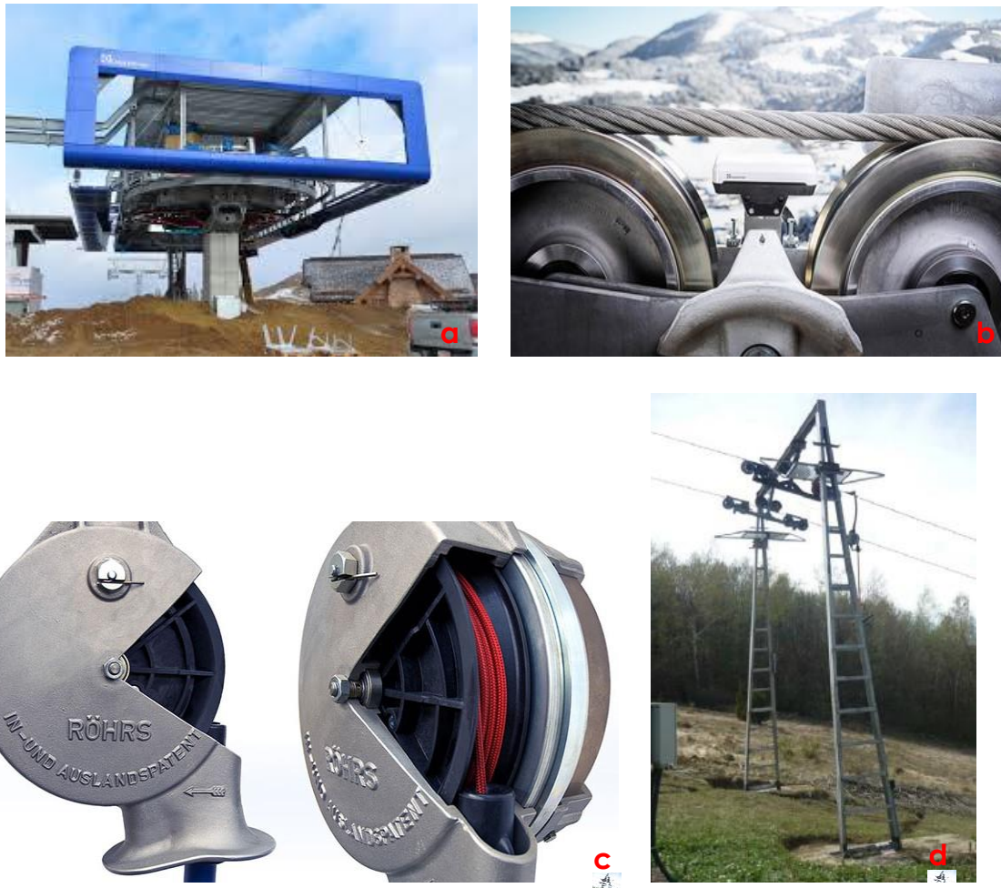
Figure 48: propulsion station (a) ,wire-rope clips (b), towing unit (c) and track supports (d) [29][30]
