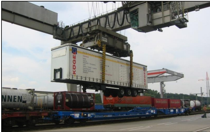
Figure 8: Transshipment of a craneable semi-trailer with help of a gantry crane
