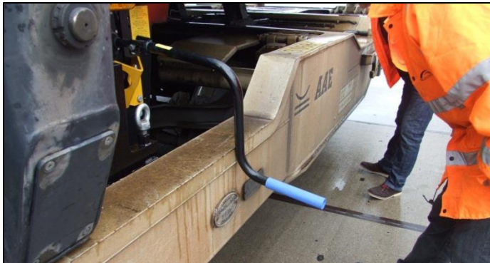
Figure 26: Blockage of the crank after loading the semi-trailer
