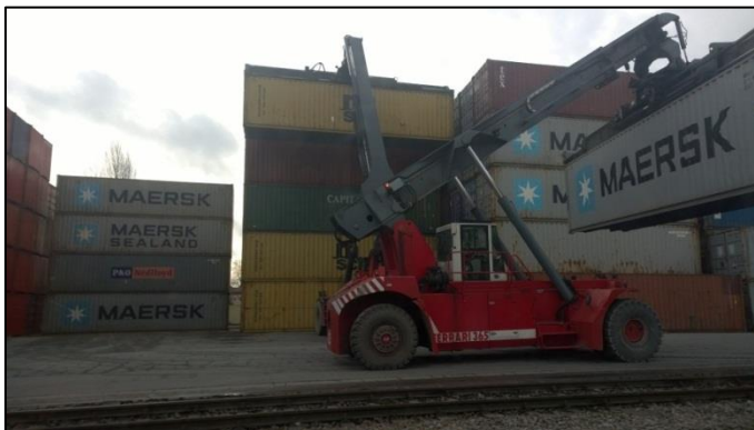
Figure 9: Transshipment of a container with a reach stacker
